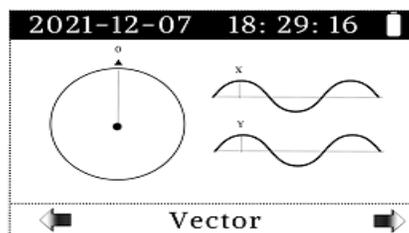
6. Move the hook of the Y-type detector to the third energized wire. The Y-type detector glows a constant red LED light. The handset main interface receives the signals and displays a new **Phase**, which is 240 degrees.
