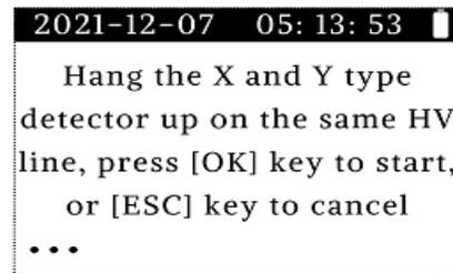
1. Attach the hooks of the X-type and Y-type detectors on the same power line.
